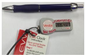
As noted previously, one of the ways that attendants can subvert the log-in requirements is to remove the EVV device from the home and carry it with them instead. As the picture shows, the device is very small, about the size of a USB flash drive. Ideally, the MCO provides the devices with a plastic zip tie with the MCO's name of logo.
